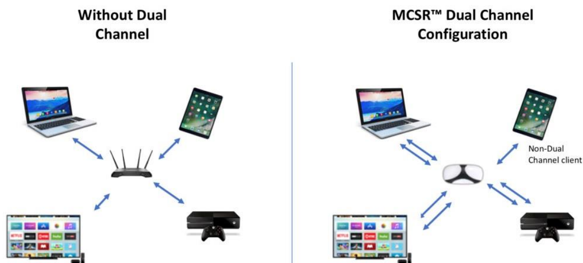
Figure 4: Internet Traffic Flow Without and With MCSR™ Powered Dual Channel Wi-Fi
